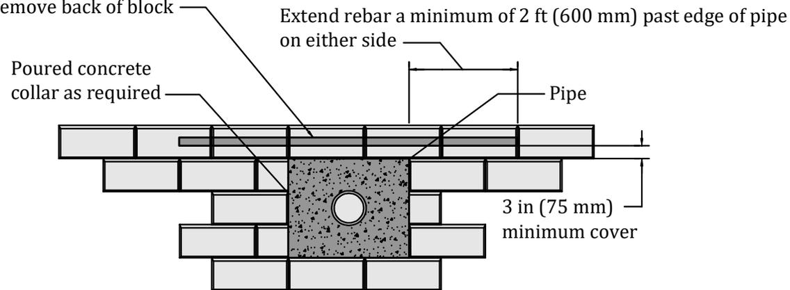
\*\* Steel reinforcement is optional and should be placed per design of engineer of record
