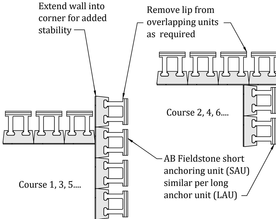
**AB Fieldstone short and long anchoring unit (SAU & LAU) corner assembly**
